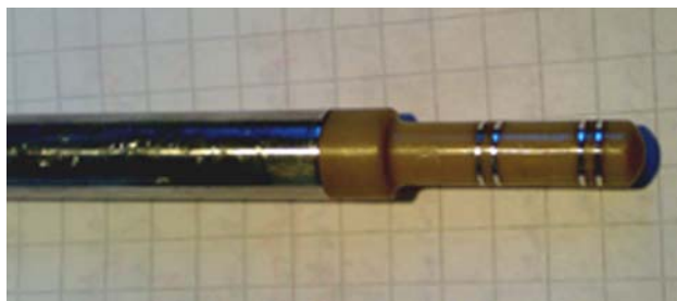
Fig. 2 The tip of the annular type dielectric probe
